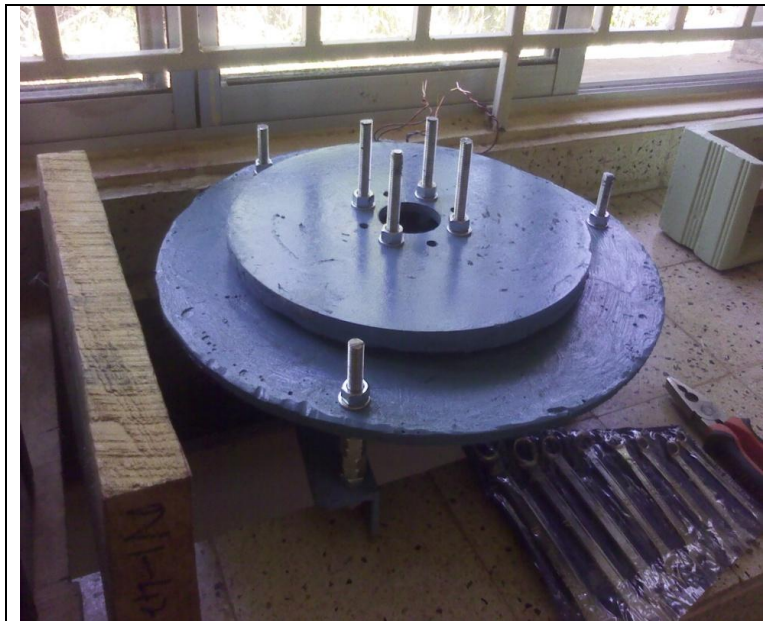
Figure 6: Assembled AFPM generator
