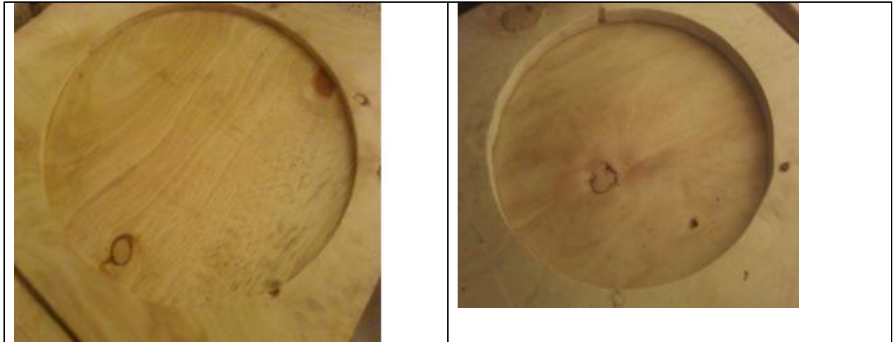
Figure 2: Finished stator and rotor moulds
