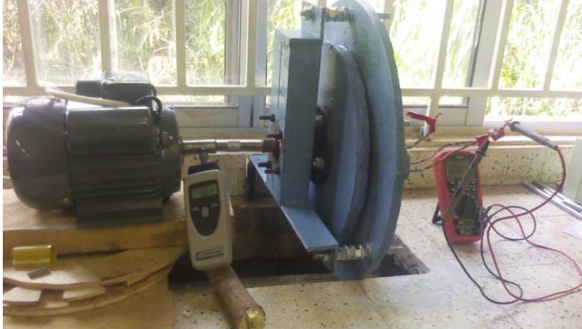
Figure 7: Generator test-set up
