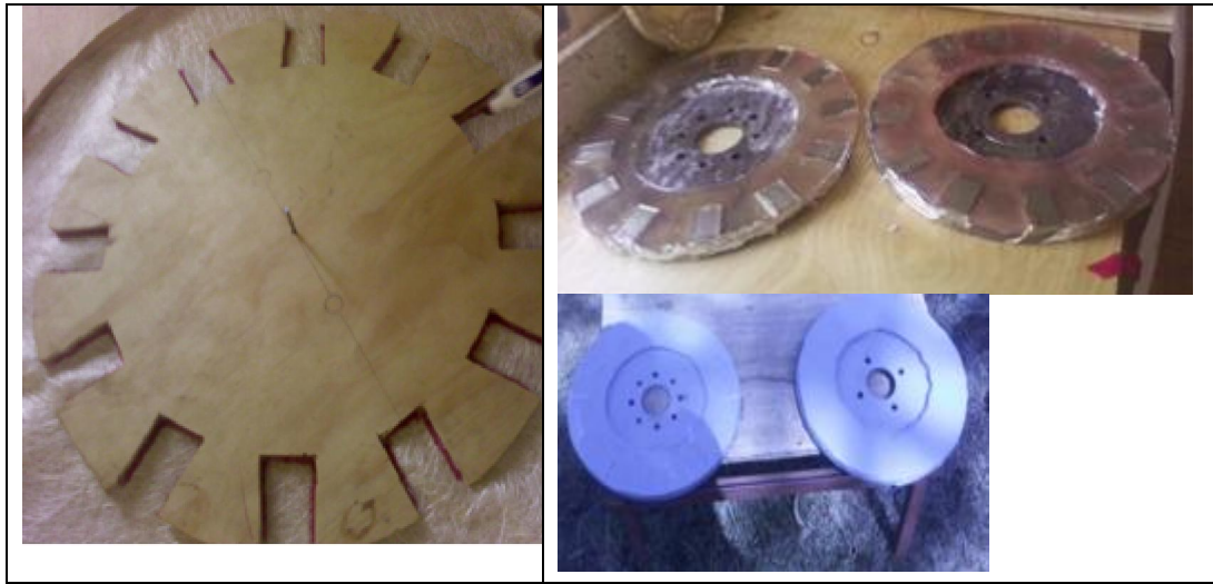
Figure 5: Magnet jig and finished rotor disks
