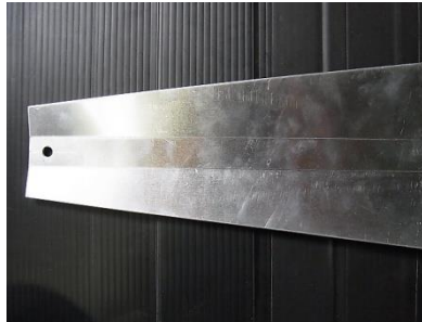
Figure 6: Type 2 of inversely tapered type aluminum curved blade
