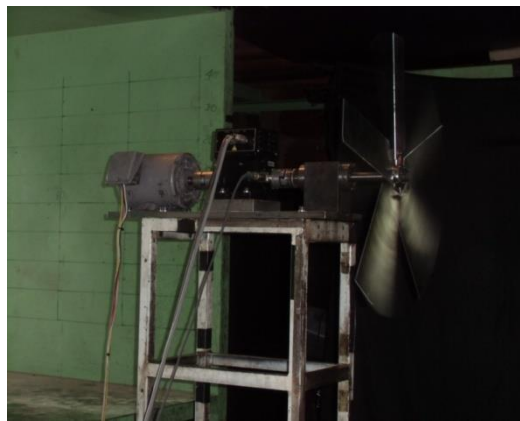
Figure 9: Turbine undergoing torque testing in the wind tunnel
