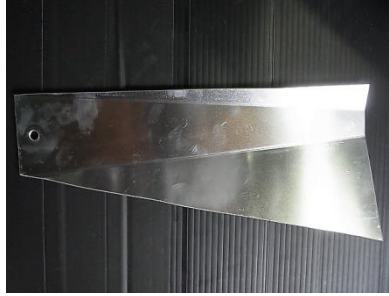
Figure 5: Type 1 of inversely tapered type aluminum curved blade
