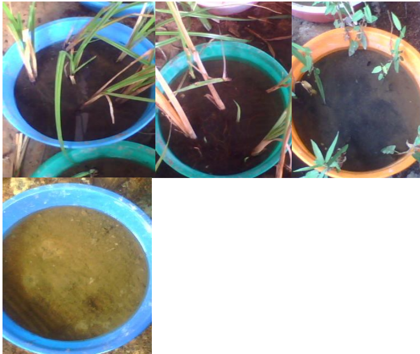
Figure 1: Experimental setup during the first experiment: reeds, cattails, smart weeds and control
